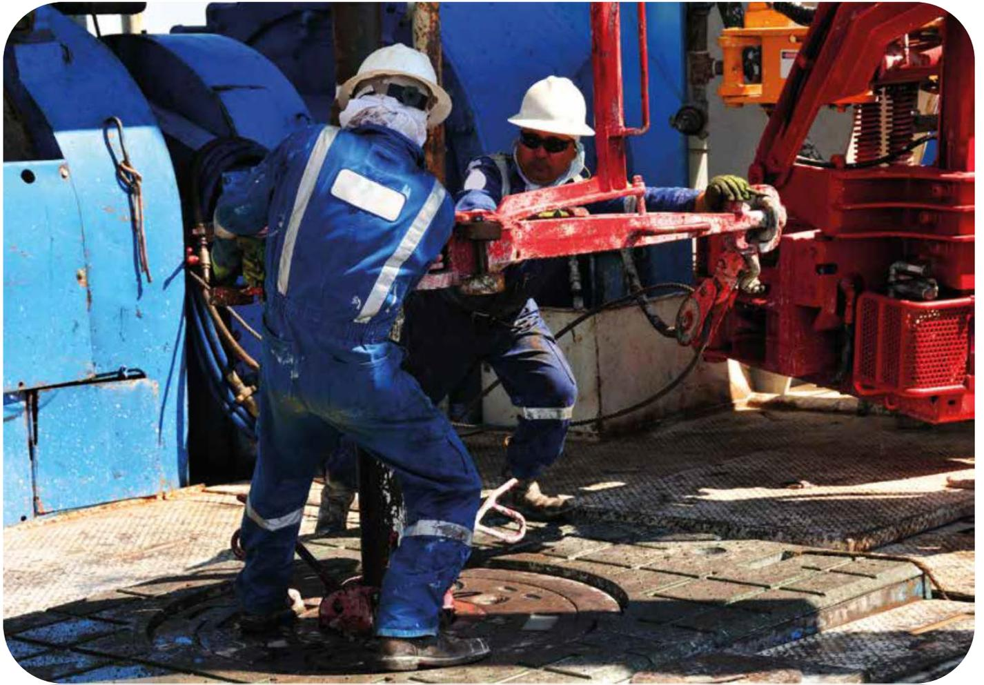
*Image of drilling rig workers making a connection during drilling operations*
